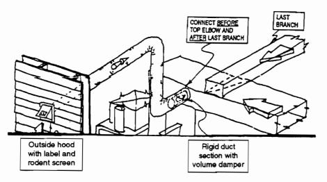
Mixing with the entire return air volume is important. Condensation on return ducts due to excessively cold temperatures has been reported where the outside air connection was to a return air plenum which carried only 1/2 of the total return air-flow.
