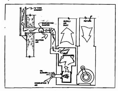
Figure 1: Natural Draft - This is traditional type of oil appliance installation. It is connected to a chimney and always considered to be type natural draft as described in 9.32.3.1(1)(c).
